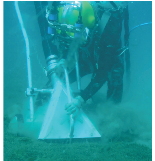
A diver guides the suction dredge over an area of exotic caulerpa. Photo NIWA
